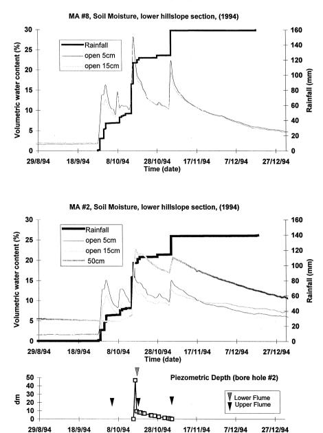
Fig. 4. Cumulative time evolution of rainfall and soil moisture, in bare ground (open) areas, at 5 cm and 15 cm depth, during the rain period of autumn 1994, at the hillslope sector (MA 8) and the lower fan sector (MA 2) of Rambla Honda. The phreatic level records are next to the lower flume and times when discharge was recorded at the flumes are indicated.
