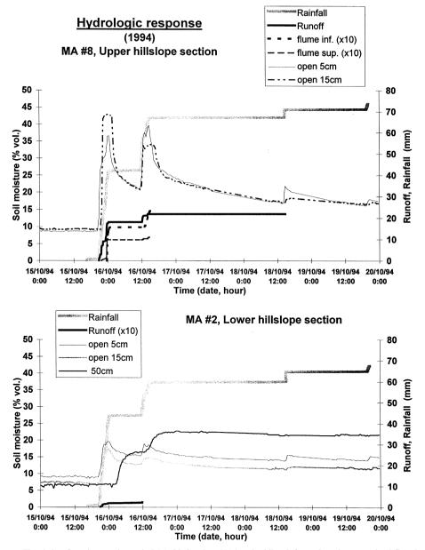
Fig. 5. The same as Fig. 4, but focusing on the period 15–20 October 1994 and adding information about overland flow in runoff plots (2 m  $\times$  10 m) and discharge at the flumes.
